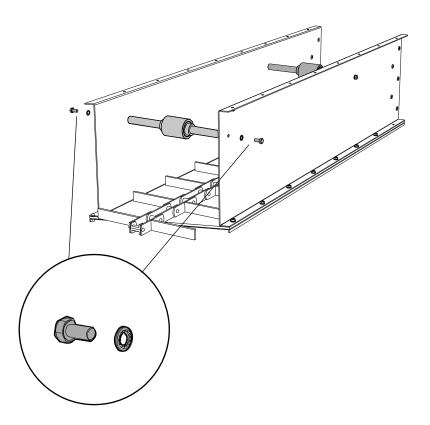
Assemble the lengths of chain in the bottom of the conveyor.
