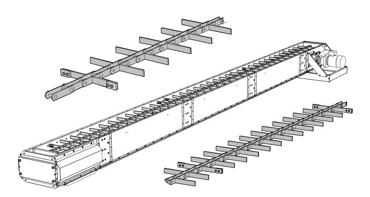
Tighten the conveyor chain with the tensioning bolts in the tail end.
